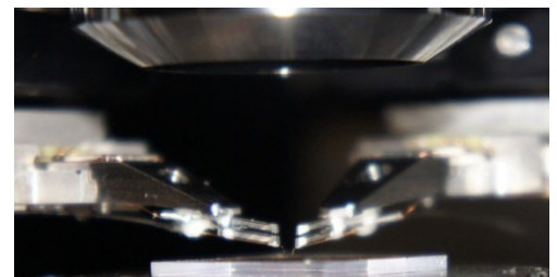
Left: Schematic for the excitation of a superfocusing surface plasmon-polariton at a metalized fiber tip by resonant coupling to a propagating fiber mode. Right: Two-tip nearfield scanning optical microscope for direct measurement of the optical near-field Green's function of photonic nanostructures.
