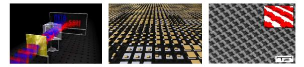
Typical inverse design process for metasurface construction: Left: A desired macroscopic optical functionality is the usual starting point. Center: This functionality needs to be integrated conceptually in a flat arrangement of nanostructures. Right: The functionality of specific nanogeometries has to be verified by rigorous simulations and technological implementations.
