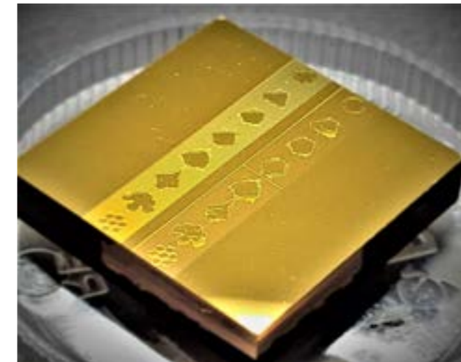
Figure 2: Phase elements fabricated at IOF for efficient demultiplexing of higher order Hermite-Gaussian modes using multi-plane light conversion.
