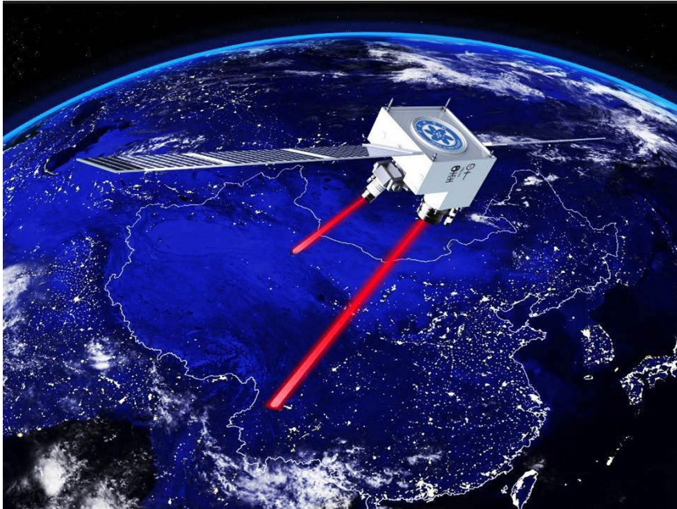
Fig. 50: Chinese Quantum Science Satellite (Micius) sends entangled photons to optical ground stations separated by 1200 km on ground © Jian-Wei Pan.
