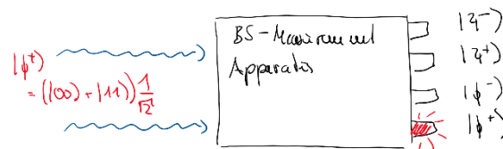
Fig. 26: Concept of a BS-Measuring device. Two Qubits enter the device and it tells you, which of the four BS the photons were in. If the photons have been in a superposition state of BSs then the resulting wavefunction will collapse into the one that corresponds to the measurement result.
