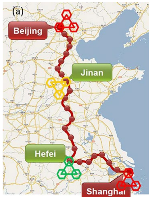
Fig. 51: The largest trusted-node network at the time of writing of this script, running over 2000 km from Beijing to Shanghai. Note, that a trusted node network does not guarantee secrecy against the operator of the network nodes.
