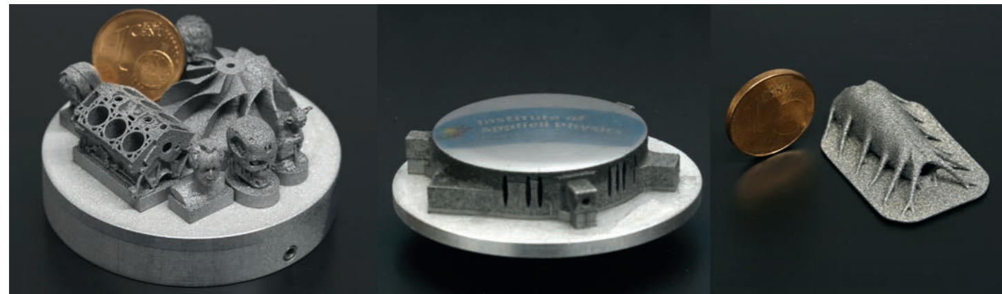
Figure 1: Complex light-weight demonstrators made of Al-40Si (left) and Al-70Si (middle and right).
