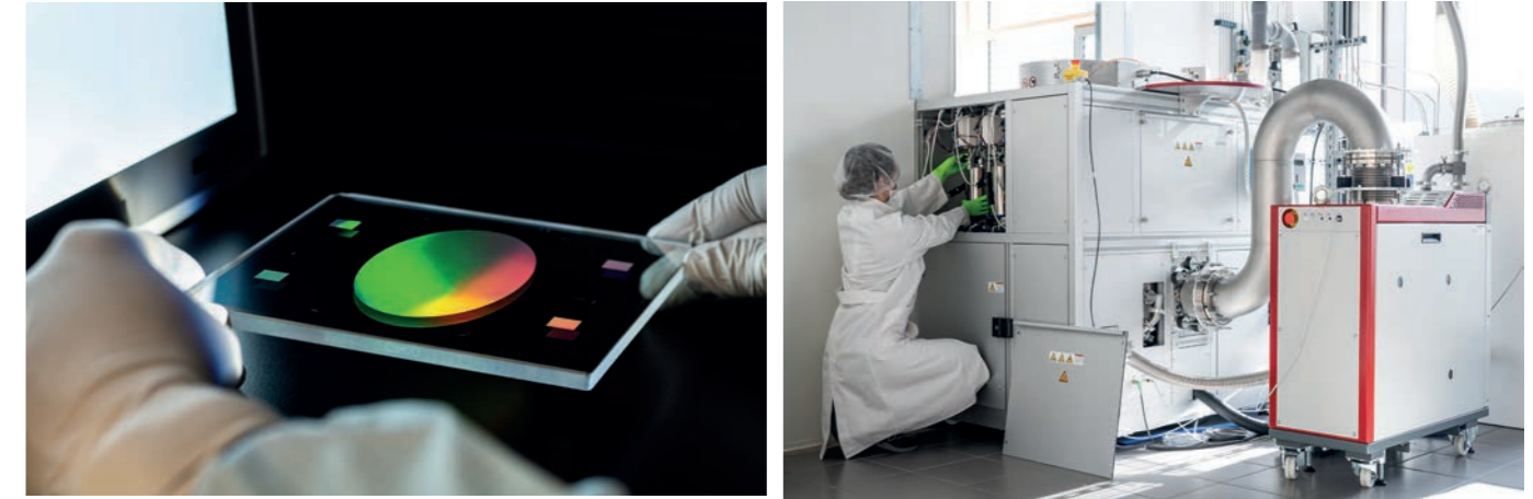
Figure 1: Photograph of an embedded grating and of the PEALD coating equipment.
