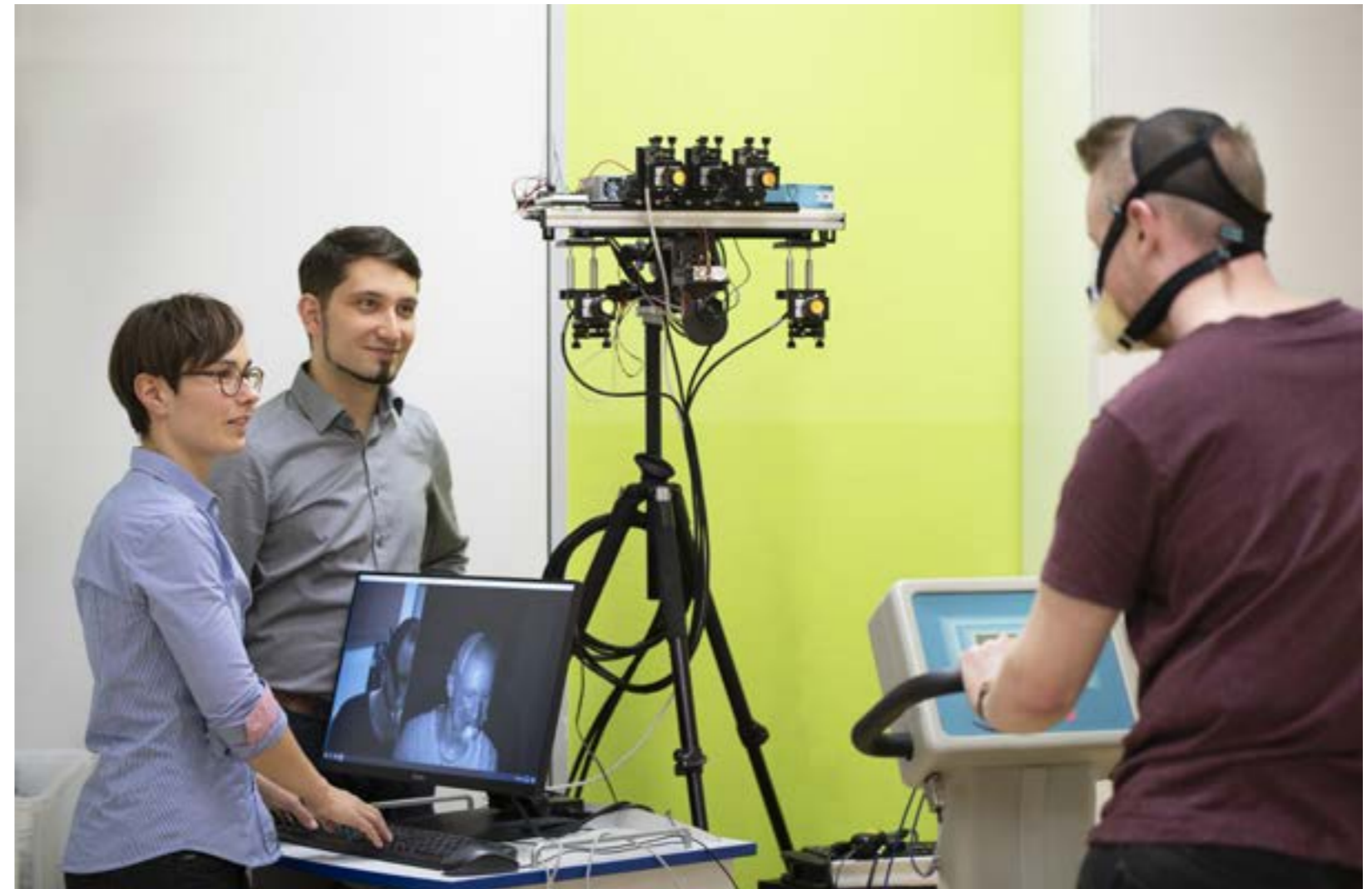
M. Nisser (Uniklinikum) and J. Sperrhake test in their NeoVitalSensor project contactless sensors that can measure vital parameters such as heart rate, blood oxygen concentration and respiratory volume by combining high-resolution 3D measurement technology and nano-optical filters.
