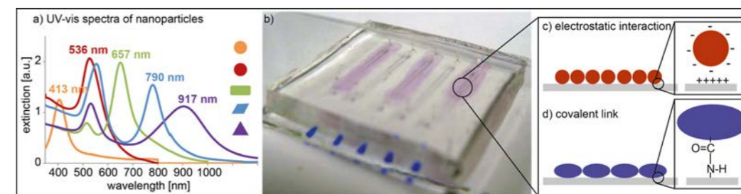
Figure 1: Spectra of plasmonic nanoparticles (a) with resonances from the visible to the near field infrared. An optofluidic PDMS chip with 5 channels (blue tick marks) bonded to a microscope slide with dense nanoparticle films (plasmonic carpets) seen as pink areas, (b) prepared by either electrostatic interaction of a positively charged surface (Aptes Silanizatio N) with the AS synthesized nanoparticles, (c) or by covalently linking carboxyl-modified nanoparticles to an aminemodified surface by carbodiimide chemistry (d).
