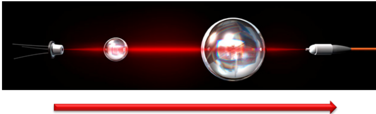
Figure 1: Unified optical modeling by field tracing: Propagation of electromagnetic fields through the complete optical system (including source and detector) by using the combination of rigorous and approximate solutions of Maxwell's equations in different subdomains of the system.
