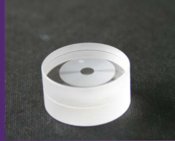
Figure 2: Bonded glass blanks after the laser welding
